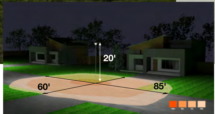
90W fixture mounted at 20' with Type III Distribution
