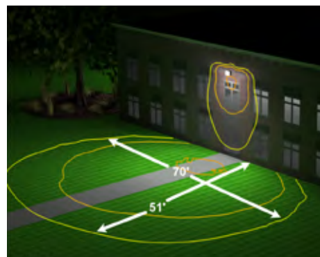
80W fixture mounted at 20' with wide distribution
