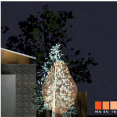
30W, 6' setback, 60° tilt, 15° beam spread
