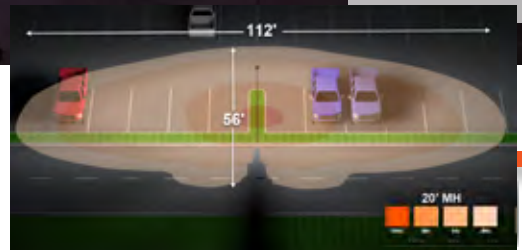
100W fixture mounted at 20' with Front Row Distribution
