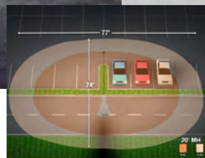
80W fixture mounted at 20' with Type V distribution
