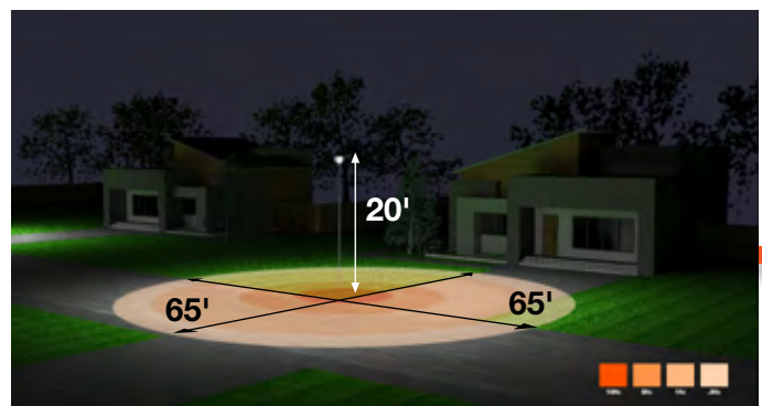
90W fixture mounted at 20' with Type V Distribution
