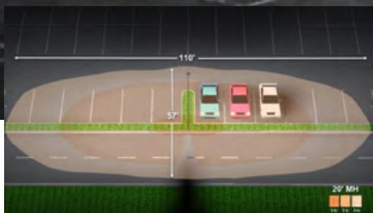
80W fixture mounted at 20' with Type III distribution
