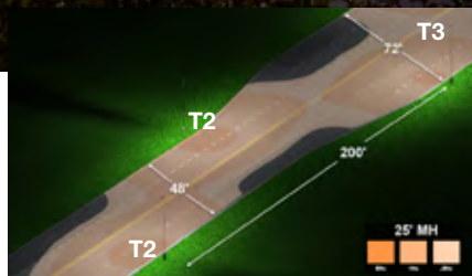
190W fixture mounted at 25' with Type II and Type III Distribution
