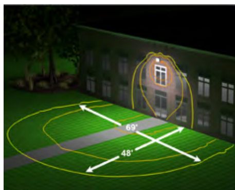
80W fixture mounted at 20' with medium distribution
