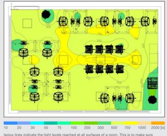
Isolux lines indicate the light levels reached at all surfaces of a room. This is to make sure that the light planning complies with norms of e.g. Em>500 lx at desk surfaces.
