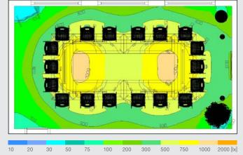
Isolux lines indicate the light levels reached at all surfaces of a room. This is to make sure that the light planning complies with norms of e.g. Em>500 Ix at desk surfaces.
